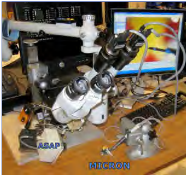
Fig. 13: Latest Micron and ASAP systems with visual tracking provided by JHU (shown on screen).
