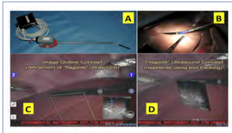
Fig. A26: daVinci Ultrasound system: A) dexterous laparoscopic ultrasound tool; B) intraoperative ultrasound scene; C, D) views through the daVinci stereo visualization system showing several video overlay concepts.
