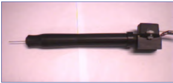
Fig. 11: First prototype Micron, an instrument for canceling hand tremor during microsurgery.
